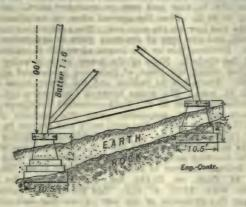
Fig. 15 .- Pedestals for Steel Viaduct.
